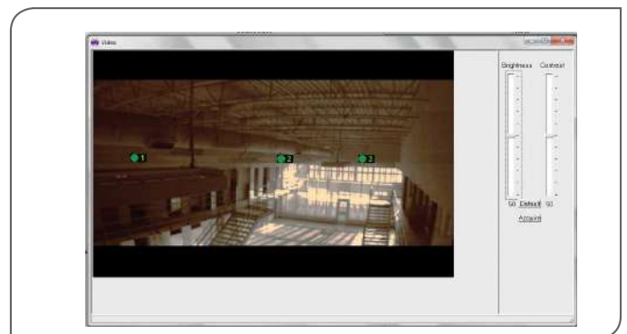
Actual view from the Imager indicating with icons the position of the various Emitters in its field of view
